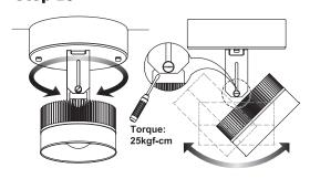
Rotate the brace to the desired orientation.
